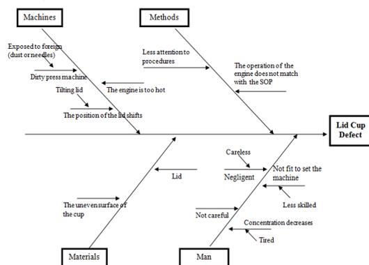
Figure 3. Fishbone Diagrams for Types of Lid Cup Defect
