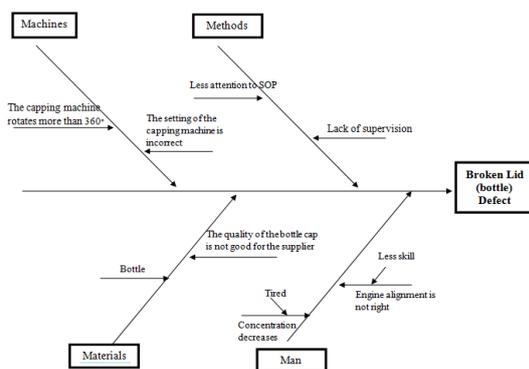
Figure 4. Fishbone Diagram for Broken Lid (bottle) Defect
