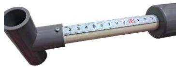
Figure 2. A pipe with a smaller diameter, functions like a piston with a scale.
