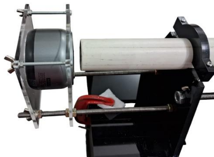
Figure 3. A Bluetooth speaker to produce sound at frequencies controlled by the Tone Generator app.
