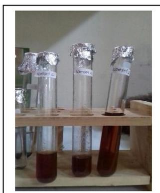
**Figure 2** Samples of used-cooking oil that have been blended for an hour to 3 hours (from right to left) and left overnight.
