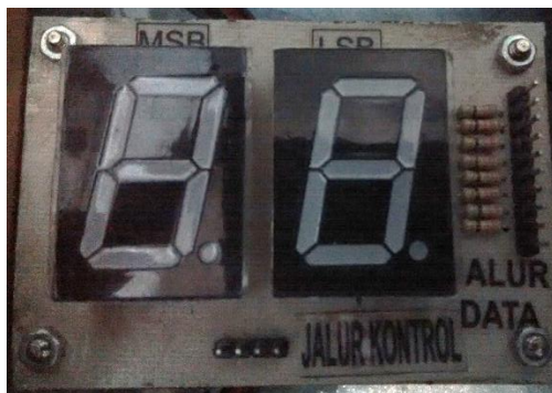
Gambar 4. Modul Seven Segment
