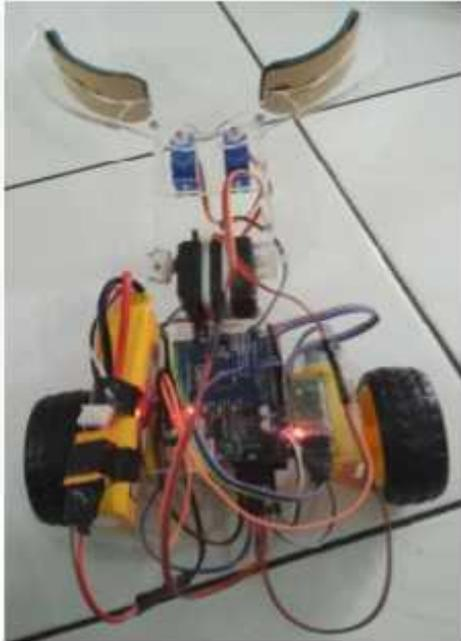
Gambar 6. *Prototype Robot Forklift*
