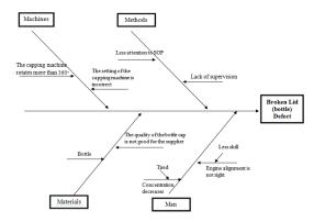
Figure 4. Fishbone Diagram for Broken Lid (bottle) Defect Based on the the fishbone diagram in
