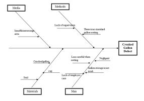
Figure 5. Fishbone Diagram for Broken Cracked gallon
