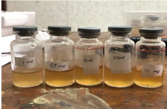
**Gambar 1.** Sintesis C-dots limbah kopi cair 1-10mL
