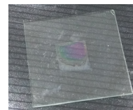
Gambar 1. Sampel compact -TiO 2 Sampel compact -TiO 2 dikarakterisasi
