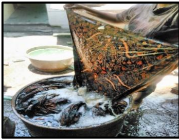
Gambar 15: Proses Pencucian Kain Batik Warna Soga Muda di Home Industry Louby Batik
